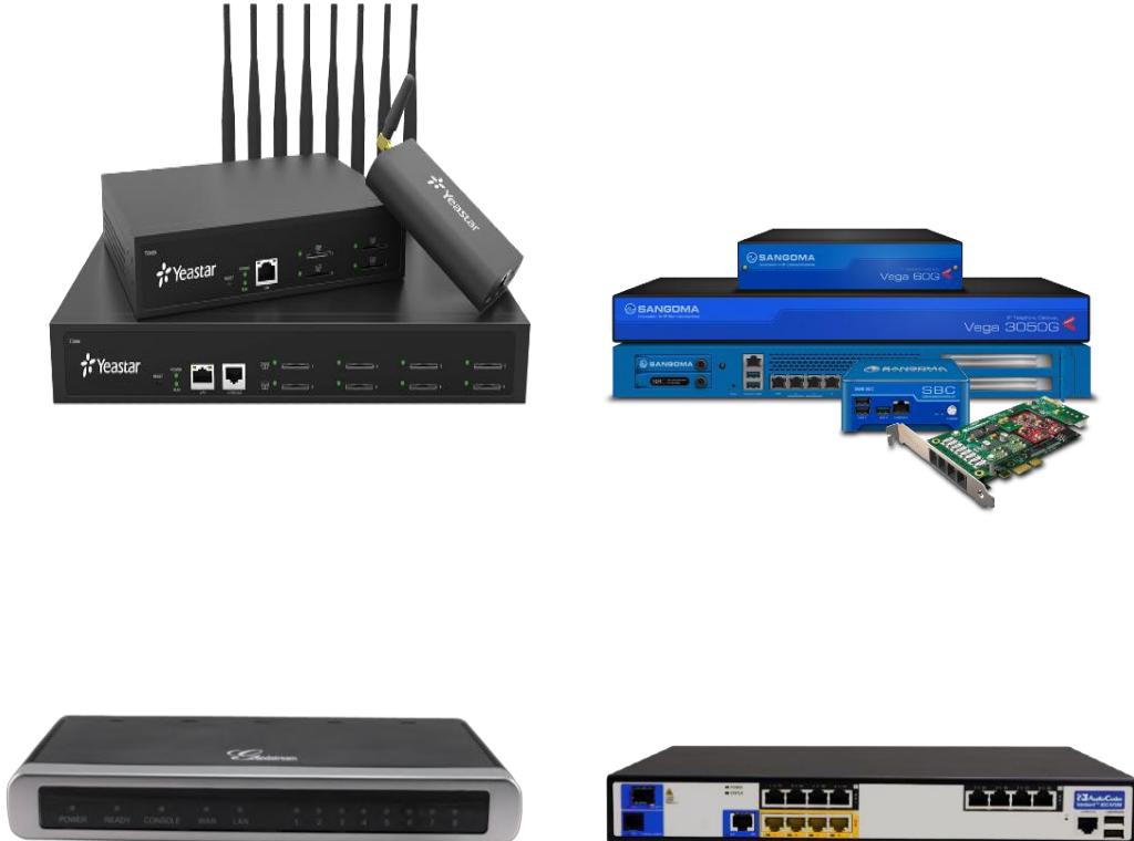
VoIP Gateway bridges the gap between FXS, FXO, PRI, BRI, GSM, 3G, 4G LTE, and IP networks to reduce operating costs and deliver the convenience.
